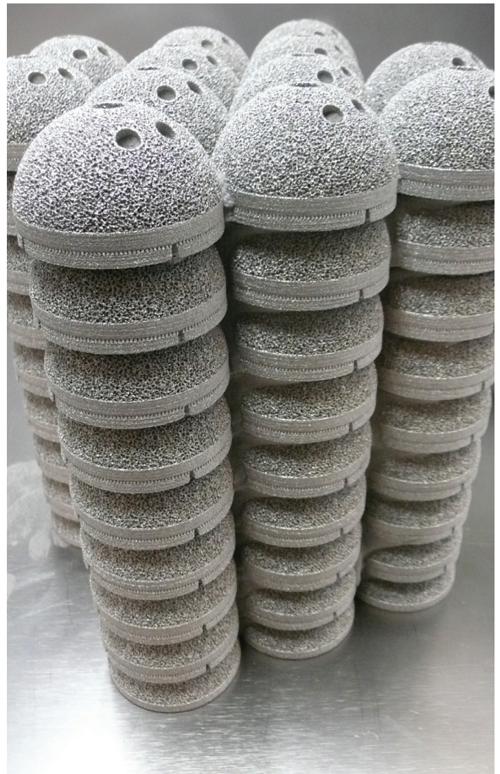
Hip cups tightly stacked with sintered powder between each part
