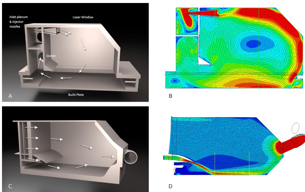
**Figure 4:** Flow concepts of GE Additive Concept Laser M2 (generations prior to Series 4) machine, (a) and b), and GE Additive Concept Laser M2 Series 4 machine, (c) and d)). Image credit: GE Additive
